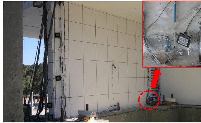
Figure 5. Web wall first story instrumentation. The top-right corner shows an LVDT in the wall/foundation interface [11].
